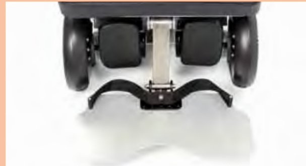
To prevent damage when colliding into an obstacle, the leg rests automatically act as a buffer.
