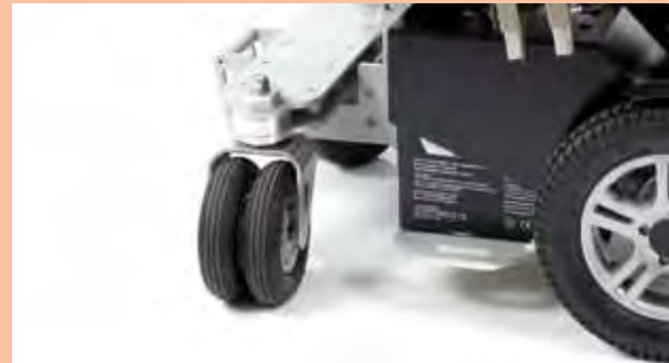
Indirect steering enables turning on the spot. The twin wheels support heavier loads and provide stability.
